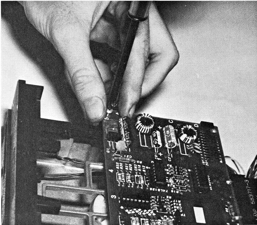
**FIG. 4-34** Remove the analog card holding screws.
