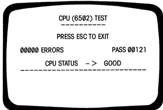
**FIG. 11-5** CPU test screen.
