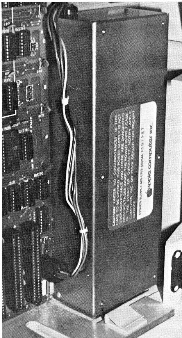
**FIG. 6-1** The power supply.
