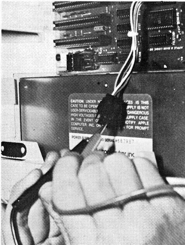
**FIG. 6-5** Checking power supply output.
