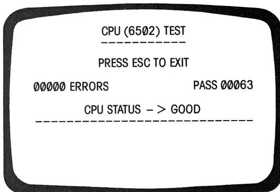
**FIG. 5-9** CPU test screen.
