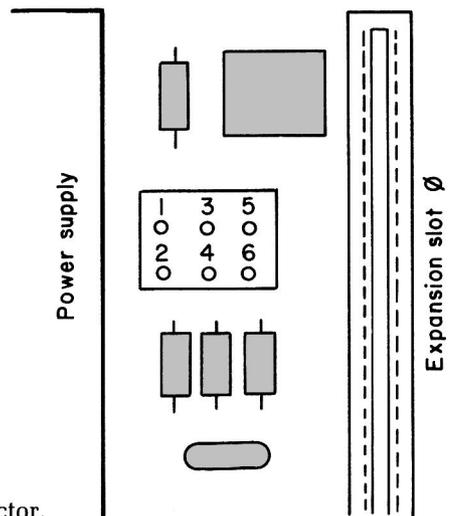
**FIG. 6-6** Pin locations on power supply connector.
