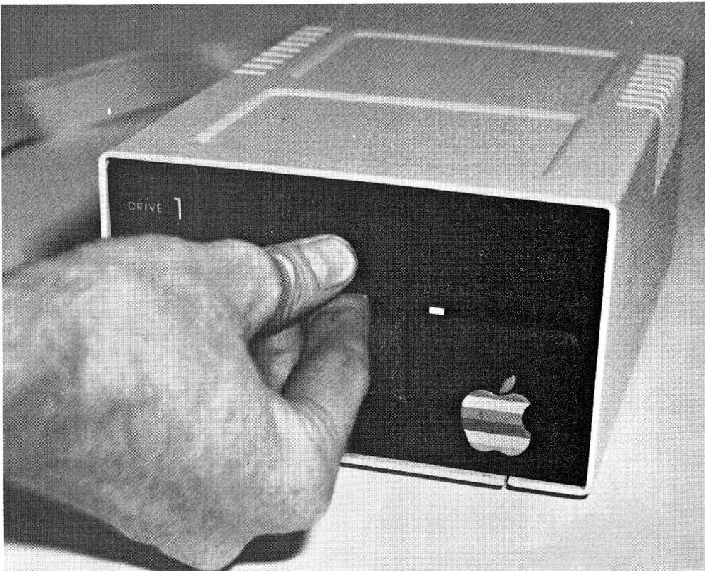
**FIG. 4-4** Make sure the door closes tightly.
