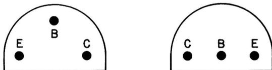
**FIG. 4-21** Typical transistor pin locations.
