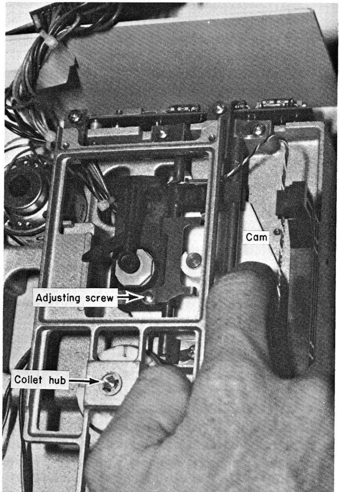
**FIG. 4-9** Adjusting screw.
