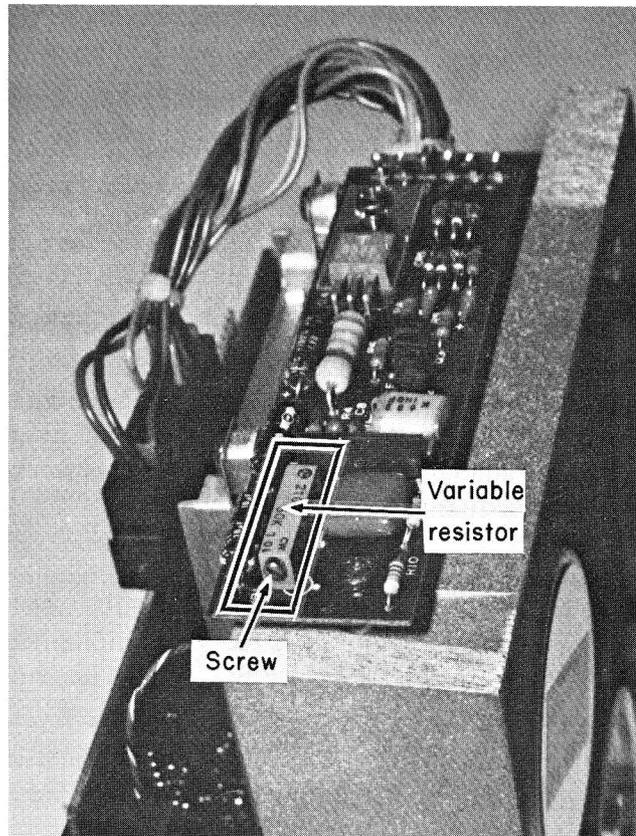
**FIG. 4-26** Variable resistor.
