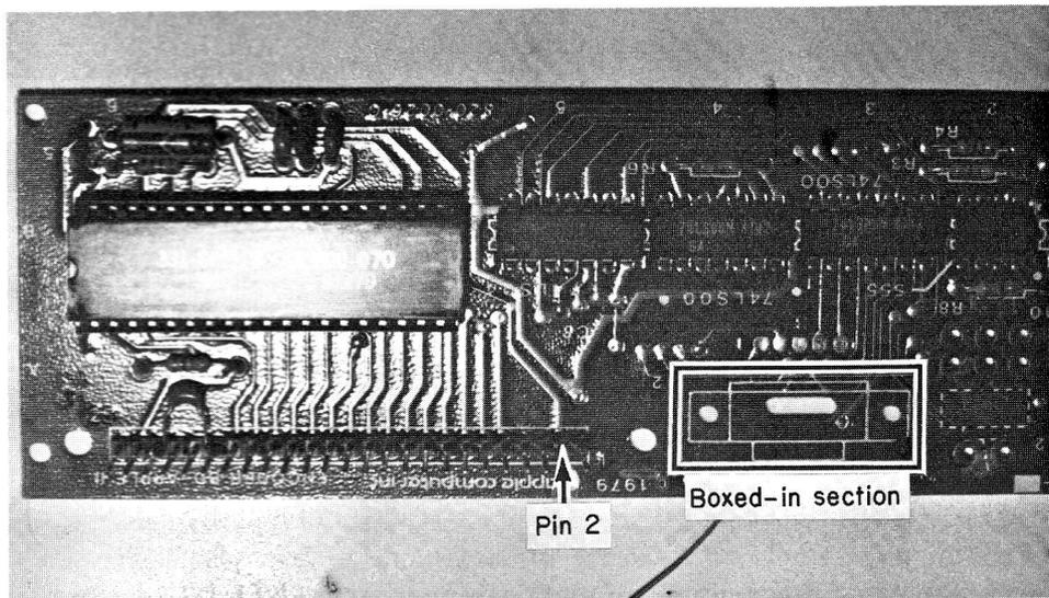
**FIG. 8-2** Location of pin 2 and boxed-in section.
