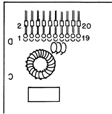
**FIG. 4-15** Pin locations on drive I/O.
