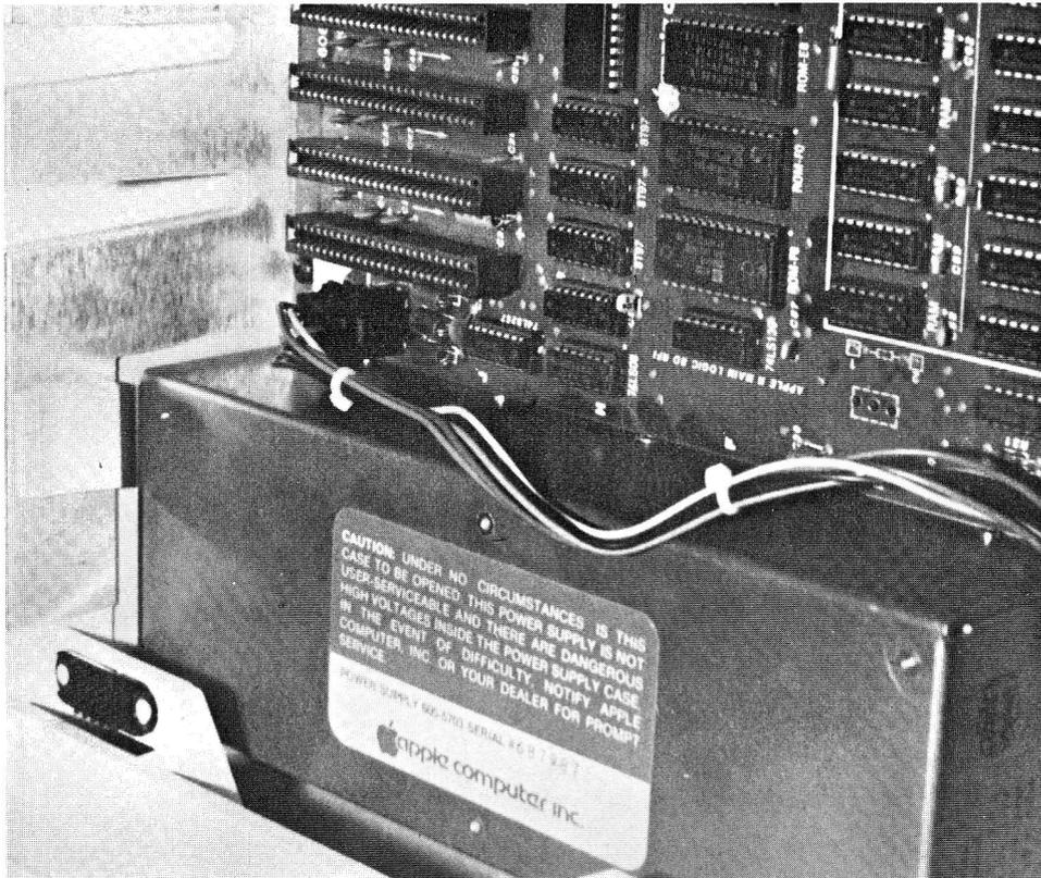
**FIG. 5-3** Location of mother board power connector.
