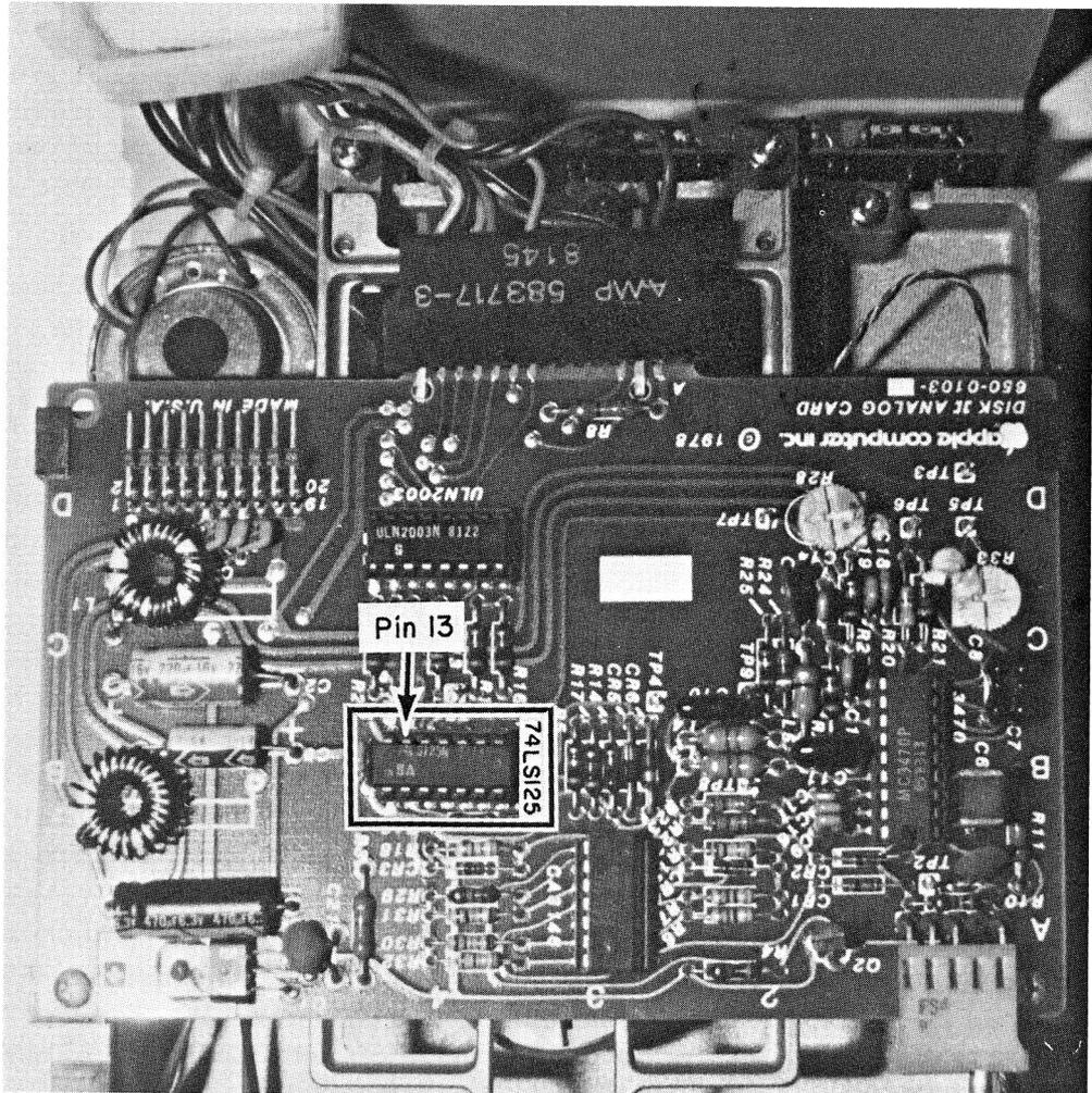
**FIG. 4-17** Location of pin 13 on the 74LS125 chip.
