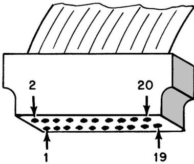
**FIG. 4-14** Pin locations on drive signal cable.
