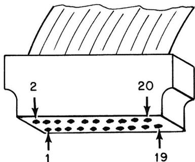
**FIG. 4-25** Pin locations on drive signal cable.
